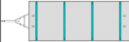
fixed floor and welded bolster
