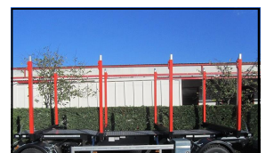
steel ExTe stakes C144
